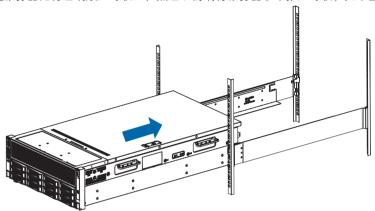
2 Locate and tighten the screws (open the small cover first) in the left and right ears of the server.
